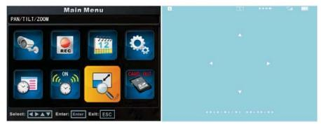
In pan/tilt /zoom menu, press enter key to enter zoom in mode, press enter again to exit zoom in mode, in zoom in mode, using key to execute up/down/left/right moving
