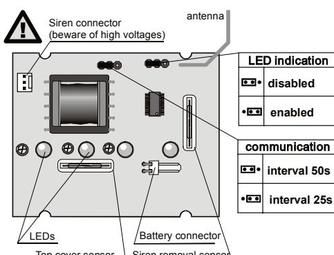
**LED ON / OFF** enables short flashes of the siren every 60 seconds (= position ON). If OFF is selected, the siren will flash only while indicating an alarm.
