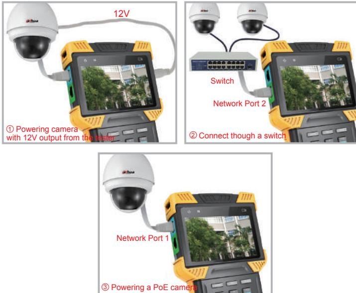
② Connect to PoE Switch and Charge the Battery at the Same Time
