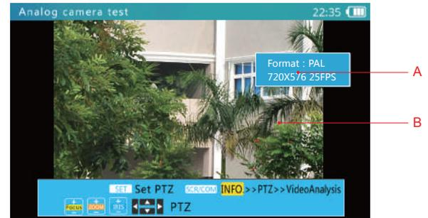
In the analog camera test interface, it can automatically identify signal format (such as NTSC, PAL, HD-CVI, HD-TVI, and AHD), resolution, and format from BNC port.
