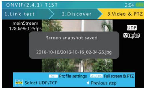
In full screen mode, you can also press A key to capture image. The example is as below:
