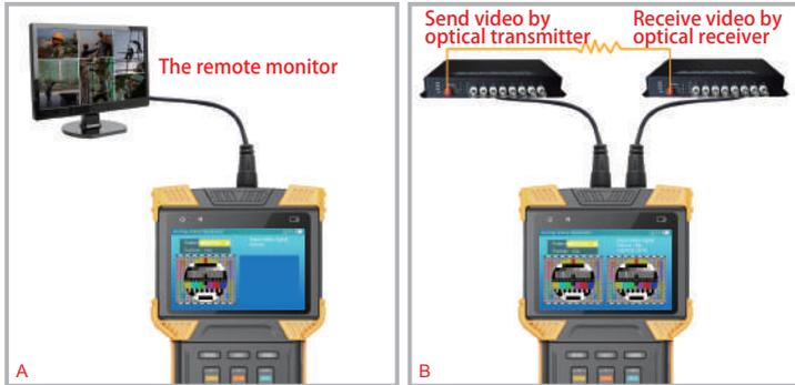
A. Transmit test video to remote monitor or DVR, and judge the transmission quality by inspecting the image.
