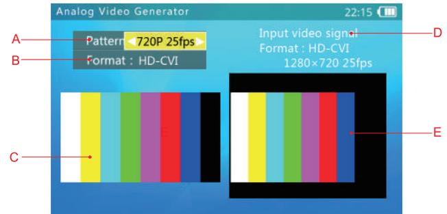
A. Test pattern: Support SD (PAL/NTSC), HD-CVI, HD-TVI, and AHD formats.
