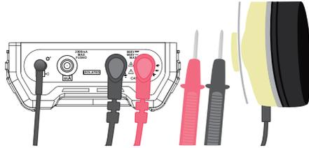
iii. Current (AC/DC) test. Connect the red probe to mA port, and the black probe to COM port.
