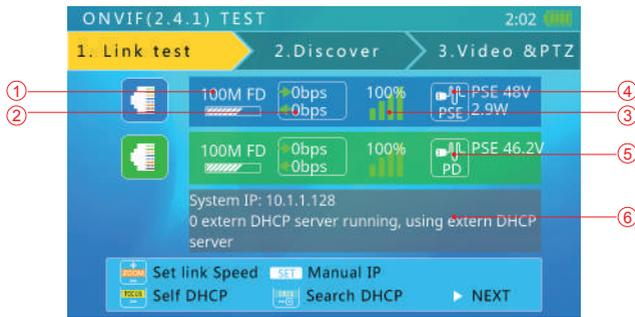
On this interface, blue bar is for network port 1 status information; green bar is for network port 2. The gray bar is IP test information. The bottom light blue bar are the operation tips.
