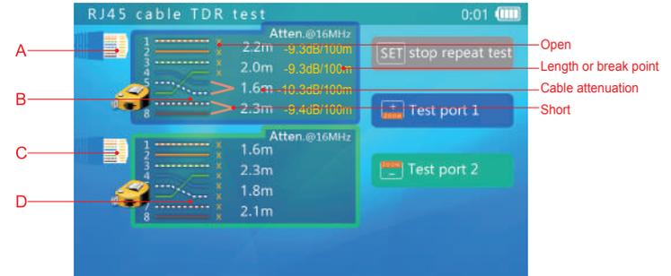
A. Network port 1 icon: A measuring tape icon flashes on the interface when a cable is being tested.
