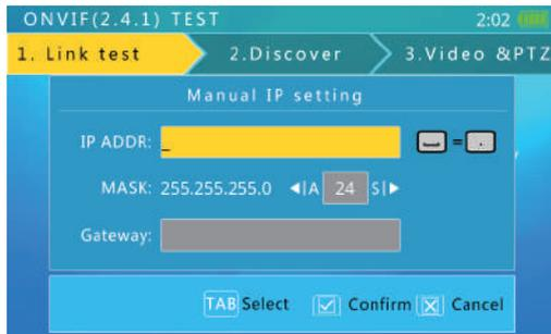
Please use the flip keyboard to enter the IP and use the A/S key to adjust the mask. To access internet, gateway is also needed.
