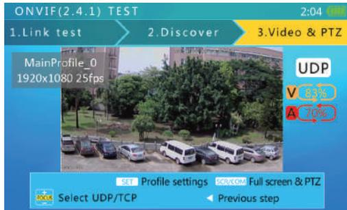
A and V mean the success rate of data transmission. V is for video and A is for audio. if the value is less than 80%, video and audio displaying might be affected.
