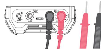
ii. Diode, and circuit on and off test. Connect the red probe to V/Ω port, and the black probe to COM port. If needed, connect an earphone to audio port in order to listen the beeper clearly in noisy environment. The earphone beeper also respond faster than the tester speaker.
