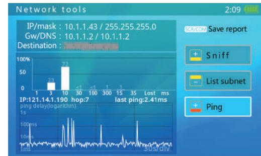
The bar chart displays the proportion of ping packets of this delay duration to the total ping packets.
