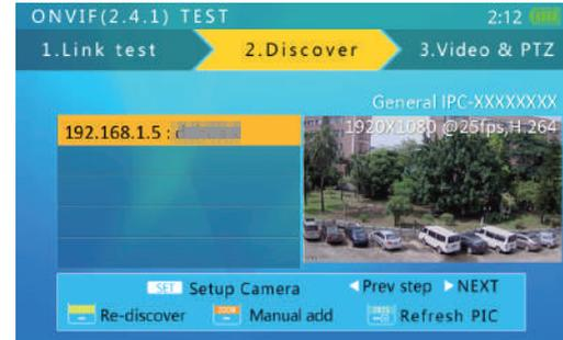
Video resolution, refresh rate, and the compression method of the camera are displayed at the top of the image.
