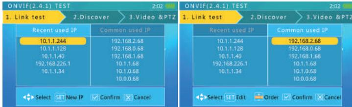
Under this mode, you can use **Recent used IP** or **Common used IP** as static IP.
